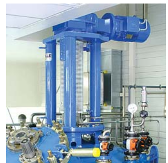
Reactor BE 8 m 3 with agitator drive TRD 500 / 7,5 / 10 kW – SX in operation at Serumwerk Bernburg GmbH
