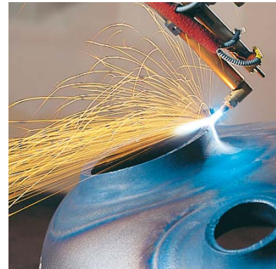
Computer-controlled flame-cutting robots guarantee high-precision synchronous cutting resulting in precise fitting accuracy of neck and nozzles
